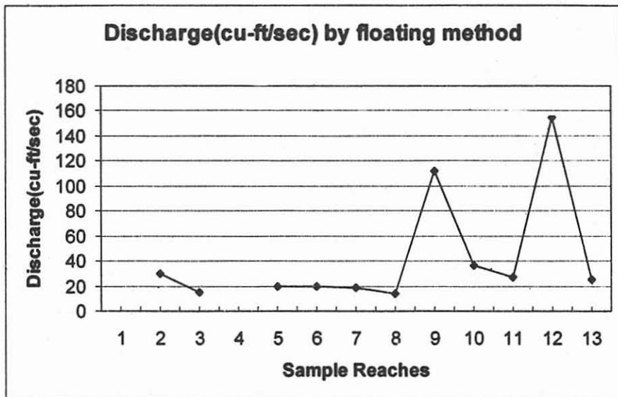
Fig. 6. Discharge of Buyo Creek in study areas measured by floating method.
